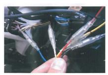
Install Red, Black, Yellow wires from the Wire Harness installed on the speed sensor wires to the wires from the Power Converter respectively.
